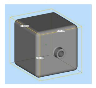
• Cube dimensions (without protrusions): 84.50 mm x 84.50 mm x 84.50 mm
