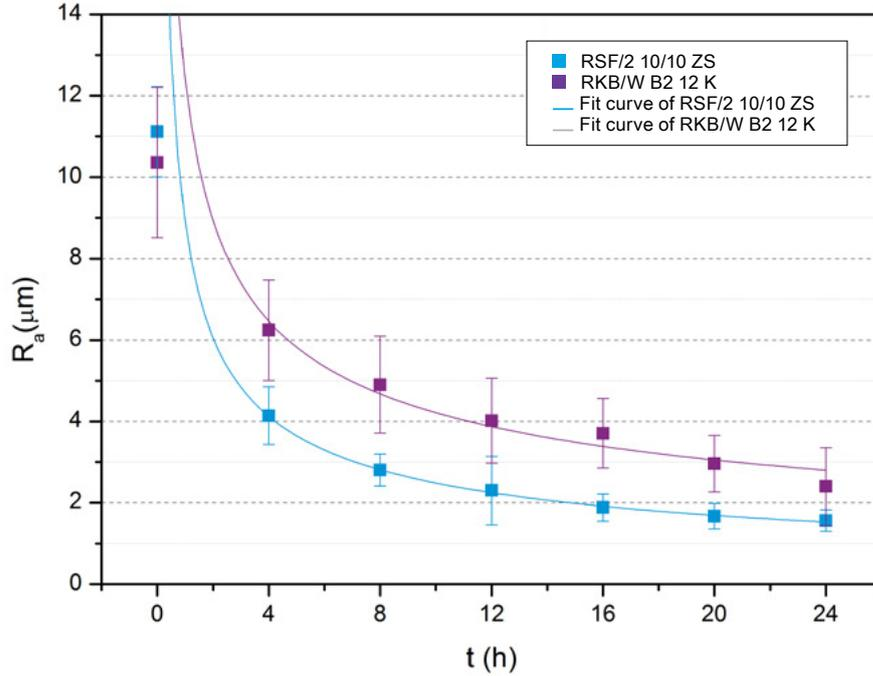
Figure 7: Surface roughness during the tumbling process with RSF/2 10/10 ZS and RKB/W B2 12 K (ceramic and plastic media, respectively)
