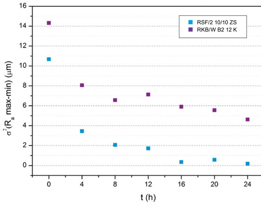
Figure 9: Evolution of the variance of difference between part surface rough
