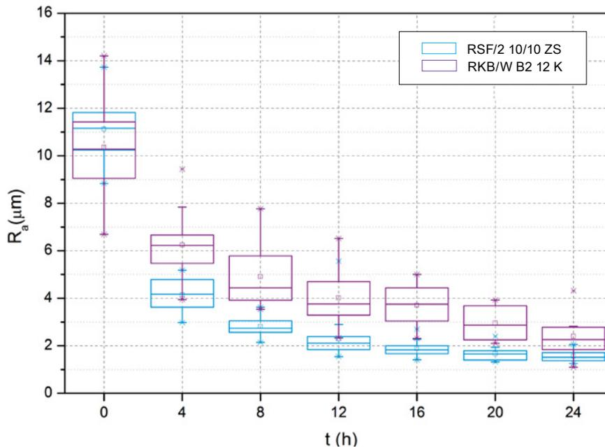
Figure 8: Bottom surface roughness box plot throughout the tumbling process with RSF/2 10/10 ZS and RKB/W B2 12 K (ceramic and plastic media, respectively)
