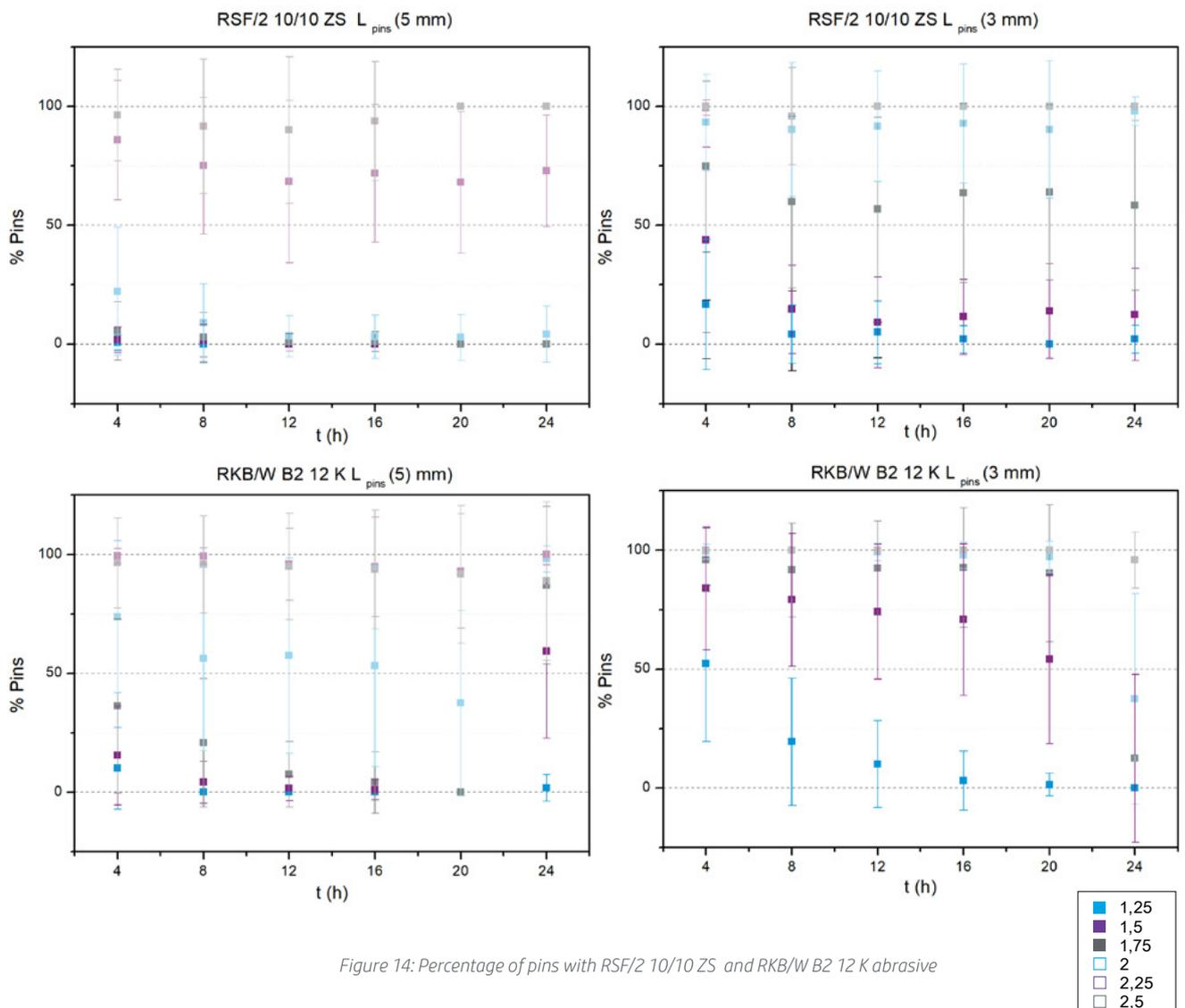
Figure 14: Percentage of pins with RSF/2 10/10 ZS and RKB/W B2 12 K abrasive
