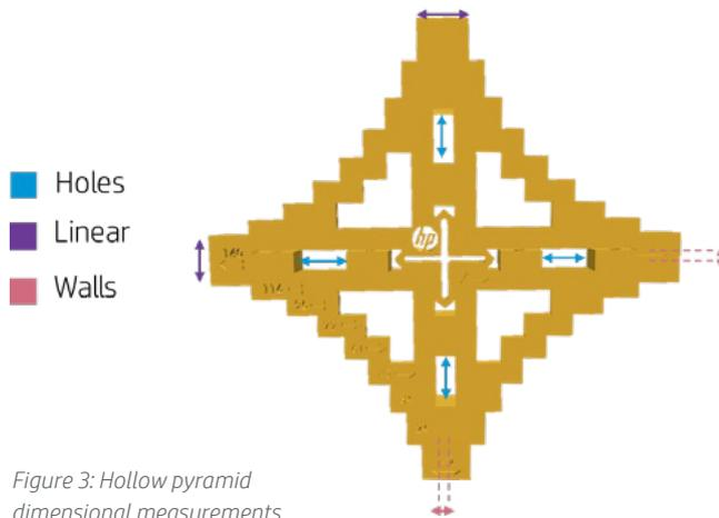
Figure 3: Hollow pyramid dimensional measurements
