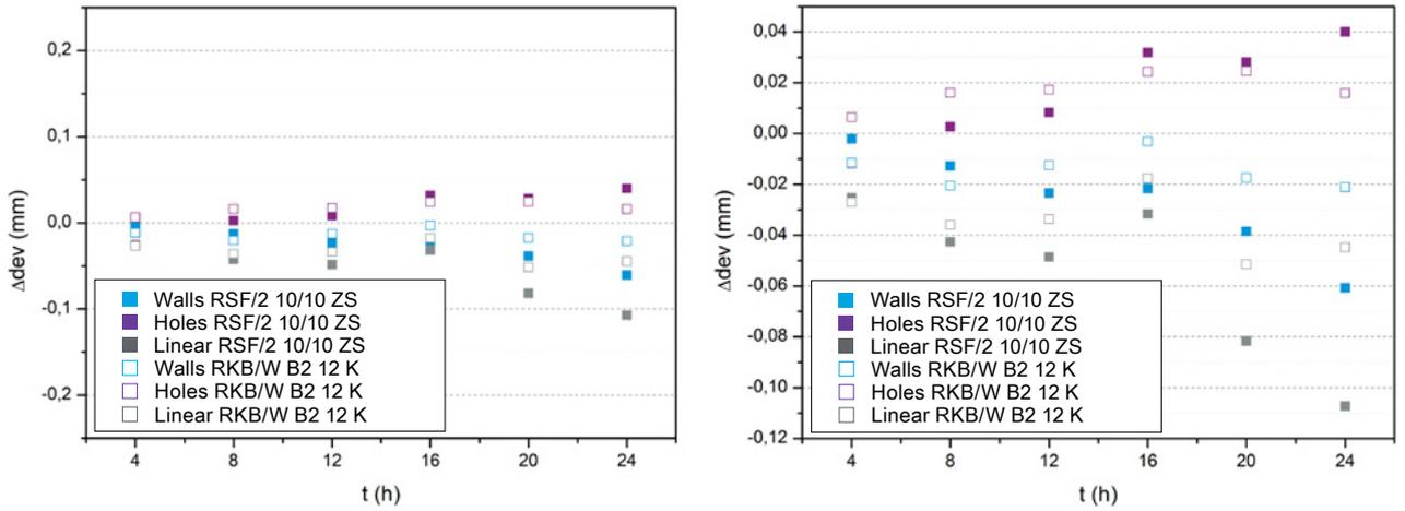
Figure 10: Dimensional variation of the tumbling process with the scale of dimensional specification of FDM parts (a) and (b) shows a zoom of the measurement.
