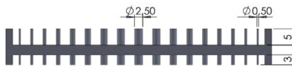
Figure 5: Pins schema (mm)
